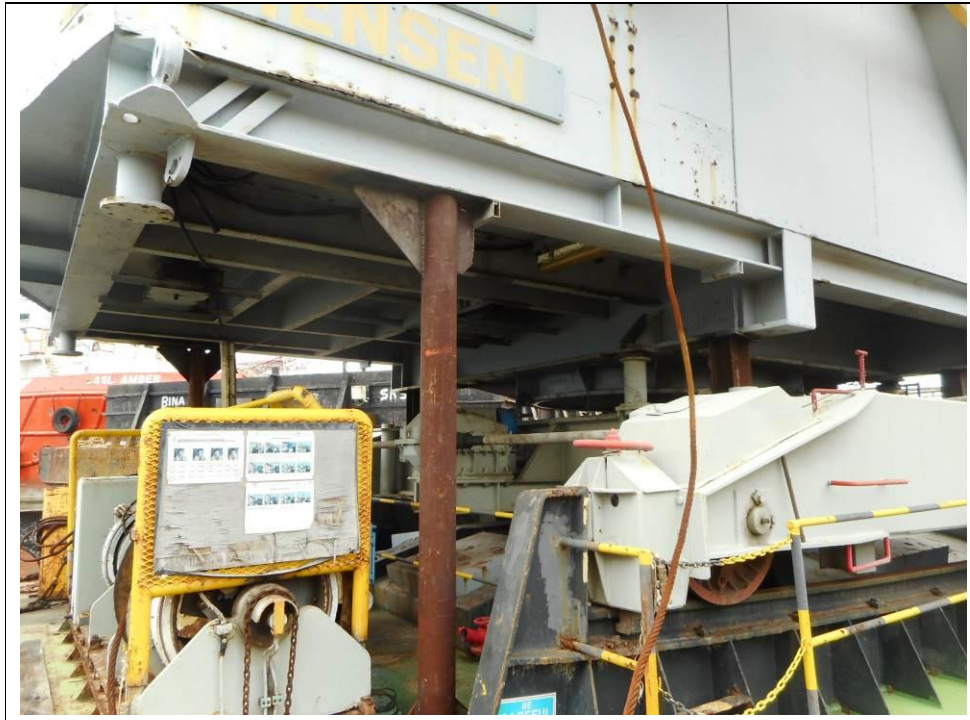
Pillar holding the crane chassis
