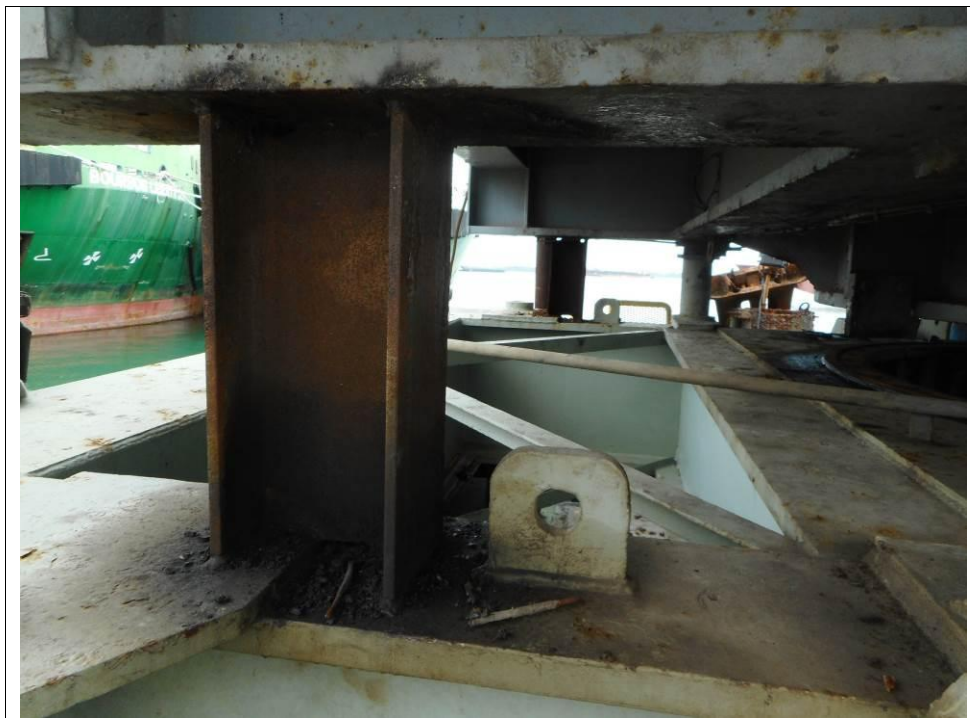
(52) H beam securing/holding the crane chassis
