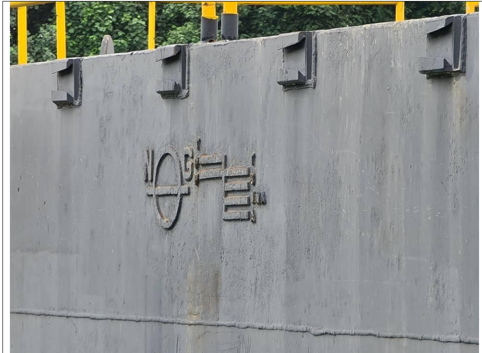
(35) Plimsoll marking / load line
