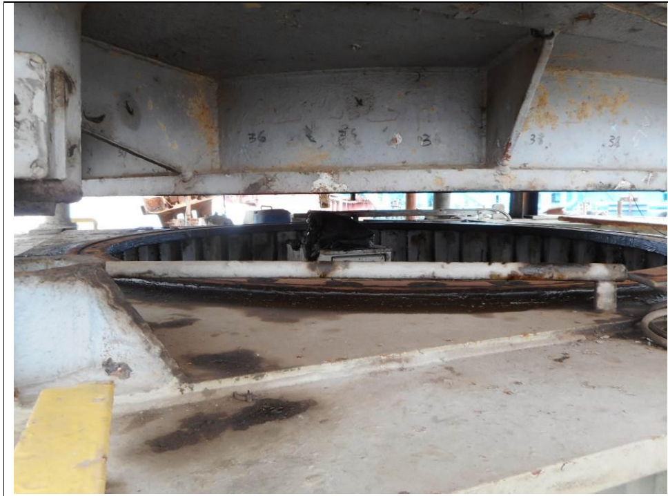
Crane turntable dismantled
