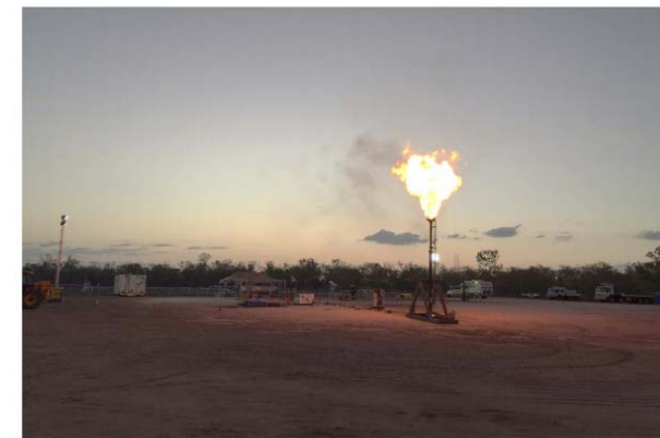
Horseshoe 4 – flare testing at 1.34 MMCFD (photo taken at 7 pm on 13 th January)
