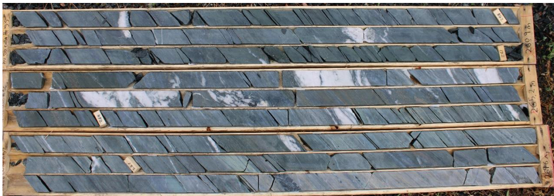
Figure 13: Vein 112 discoveries. 3m @ 7.4 g/t gold from 261m in AUDD0010. Multiple quartz-ankerite-pyrrhotite-pyrite-gold veins within high strain fuchsite, sericite and ankerite altered basalts at the contact between basalts and Temiskaming like conglomerates.
