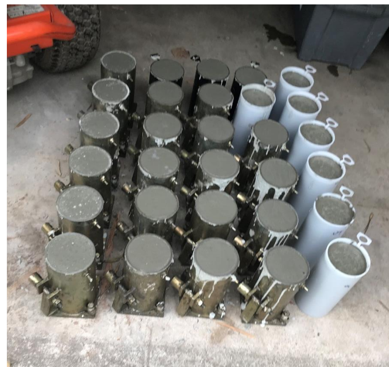
Concrete Test Pieces containing Halloysite-Kaolin Rheology Modifier Products
