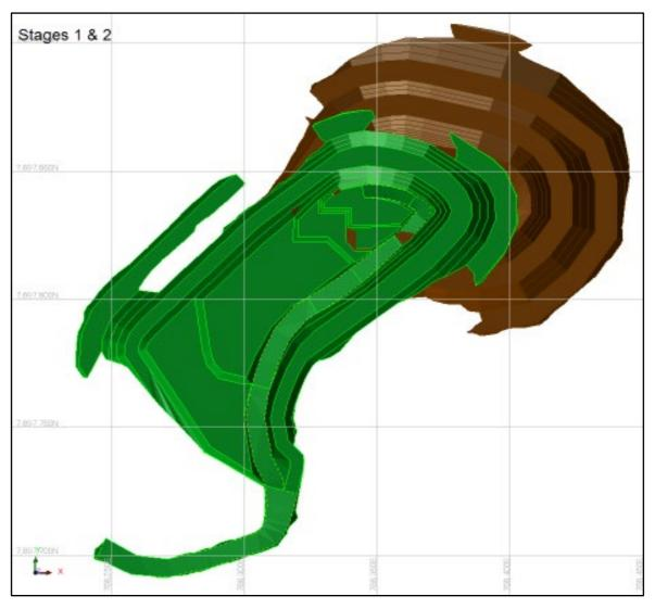
Basic pit outlines Green Stage 1 cut back which will produce around 18,000t of ore material
