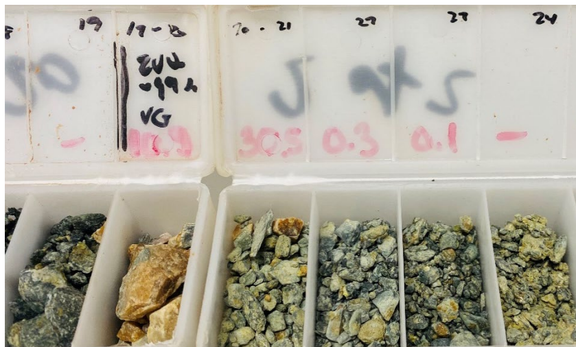
Figure 4: RC chips from MZRC022 (18-24m) showing an intercept of the lode consisting of an oxidised quartz vein from 19-21m grading 20.7g/t Au.
