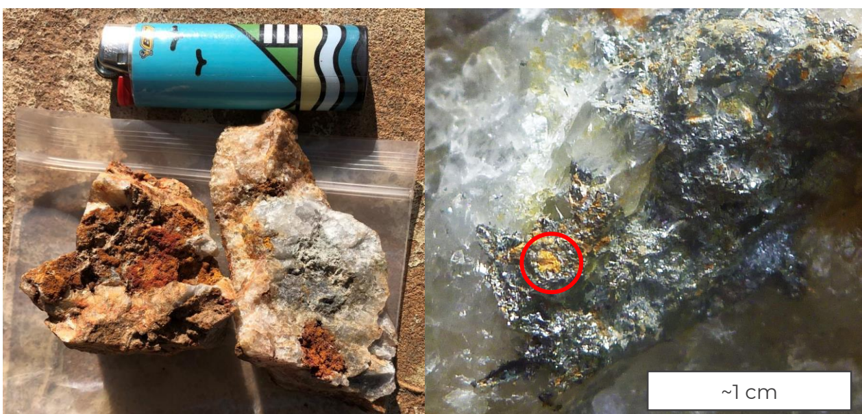
Figure 2 Covidicus West Prospect mineralisation style. Left: irregular limonite and arsenic oxide filled pits in quartz vein, weathered from sulphides. Right: arsenopyrite with small grain of free gold (circled).
