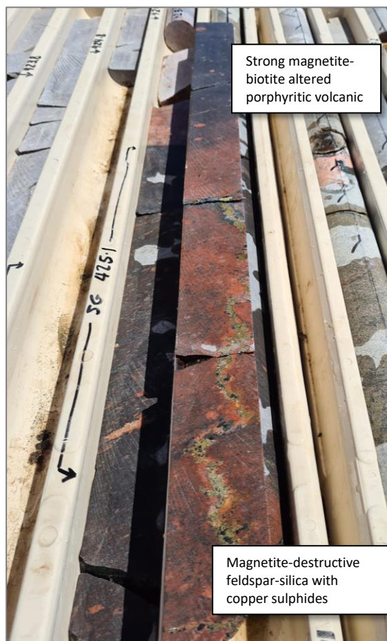
[Figure 10] Corkwood Project: Porphyritic volcanic rock showing early magnetite-biotite alteration (black colour at the top) demagnetised by red feldspar-silica alteration and associated chalcopyrite (weak magnetite) veining.
