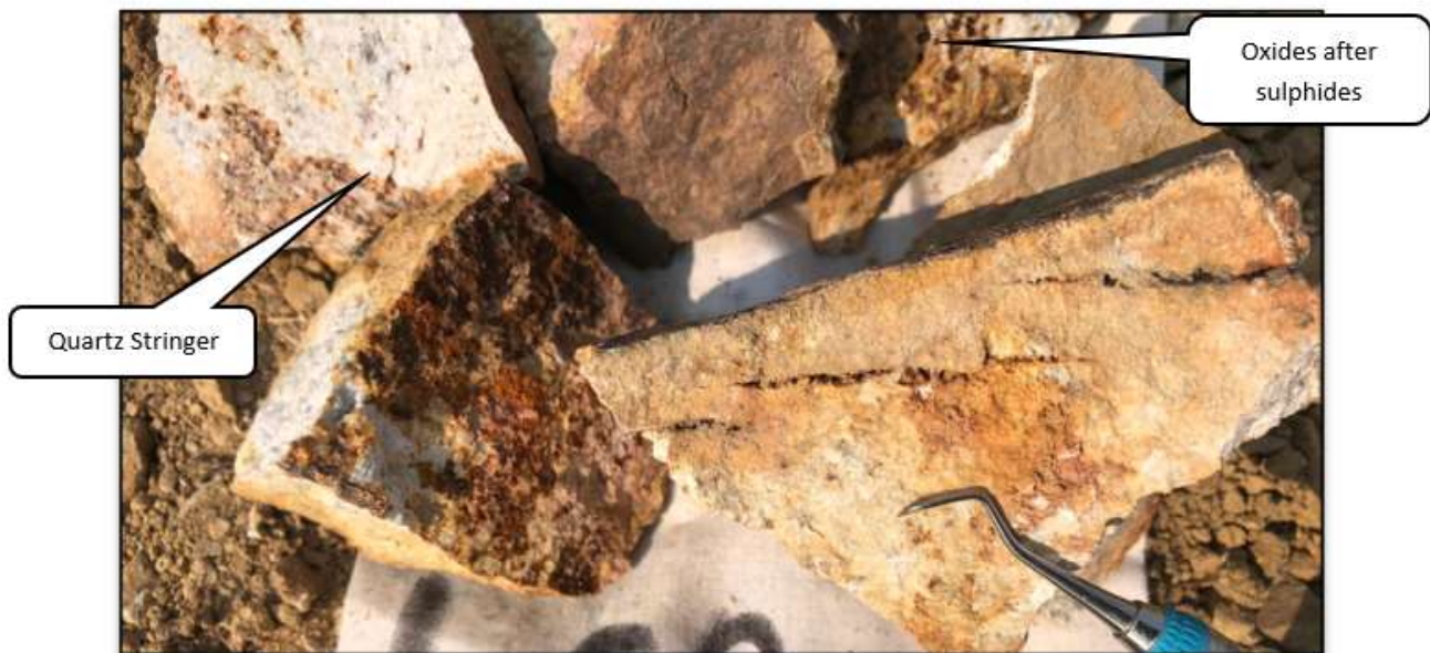
Figure 5: Outcropping altered felsic intrusive rocks with quartz stringers and oxides after sulphides, exposed during road construction
