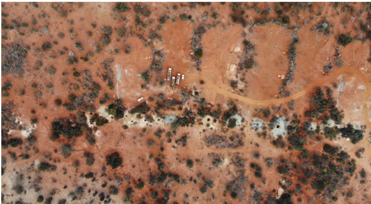
Figure 10: Drone image (north to the right) showing historical workings at Metzke's Find including additional workings to the south (left side of the image). The rig is on drill hole MZRC013 in this photo.
