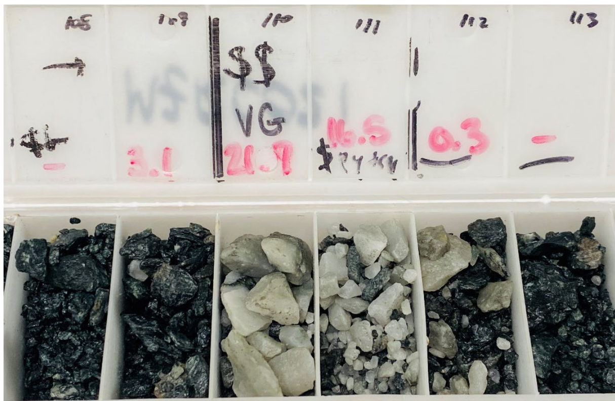
Figure 3: RC chips from MZRC021 (107-113m) showing an intercept of the lode consisting of a sugary quartz-sulphide vein within a biotite altered structure from 108-111m grading 13.8g/t Au.
