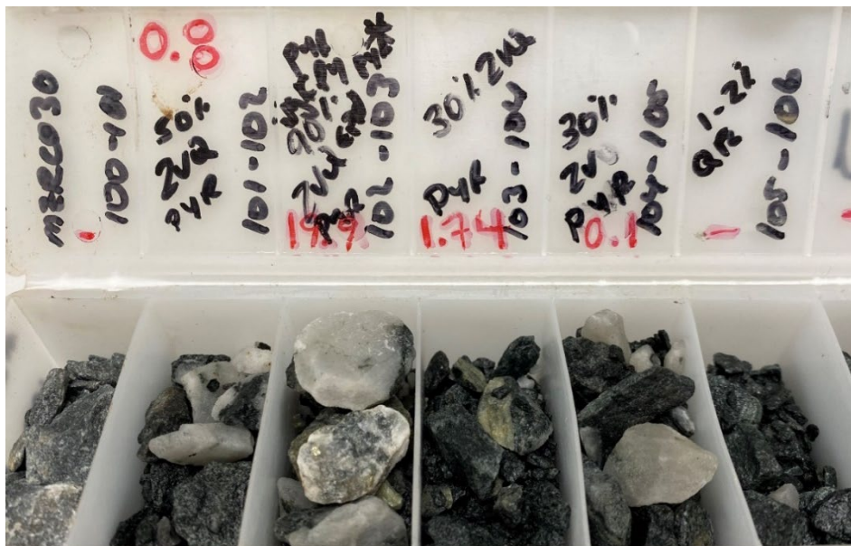
Figure 4: RC chips from MZRC030 (100-106m) showing an intercept of the lode consisting of sugary quartz-sulphide vein within a biotite altered structure from 102-104m grading 10.8g/t Au
