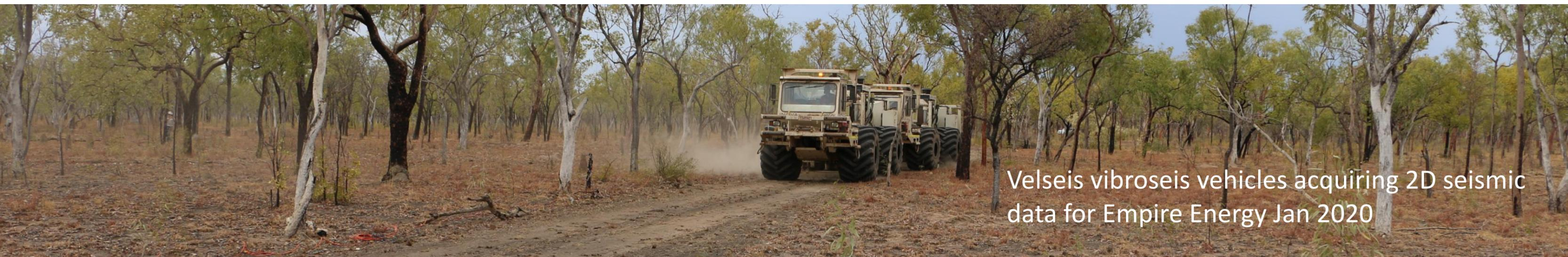
Velseis vibroseis vehicles acquiring 2D seismic data for Empire Energy Jan 2020
