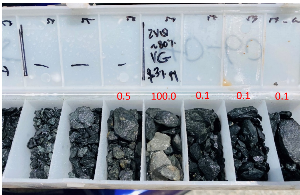
Figure 1: Chip tray from LMRC005 53-60m showing the high-grade lode from 56-57m.
