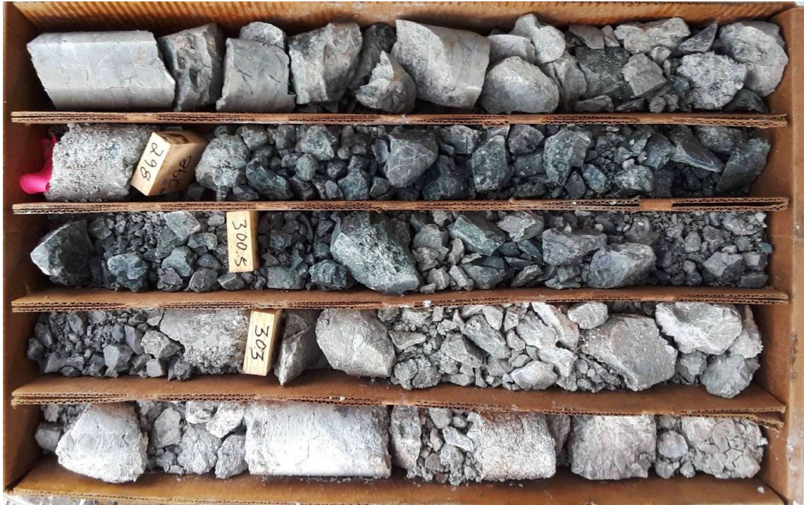
Figure 5. Highly fractured, Intensely silicified and bleached metasediments 269.6ft to 306.5ft (82.2m to 93.4m)
