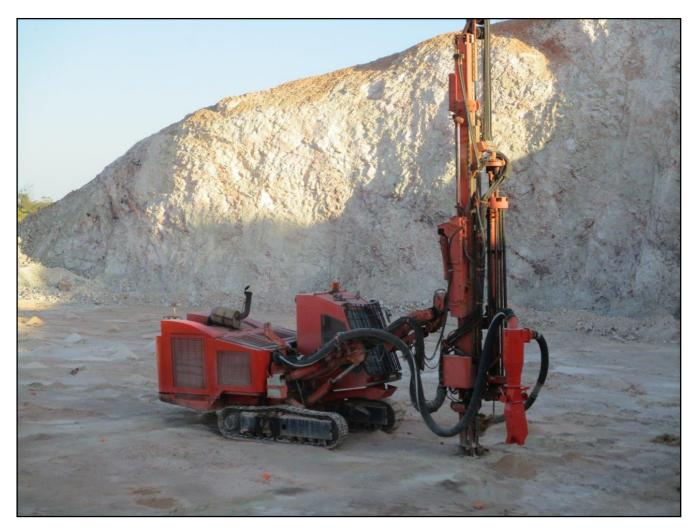
Blast hole drilling in preparation for initial blast – 16/10/2020
