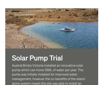
electric pump with zero fuel costs, no carbon emissions and no requirement to install energy infrastructure.
