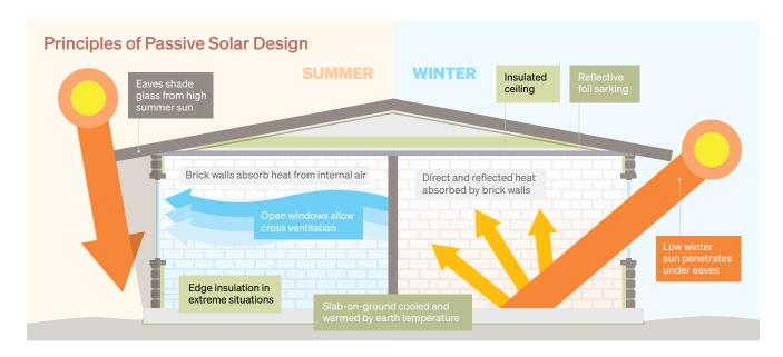
Brickworks boasts a number of buildings products that contribute to improvements in thermal performance. Bricks provide human thermal comfort, and are high density materials, meaning they have an ability to effectively absorb and store heat energy keeping your home cooler in summer and warmer in winter. This is something lightweight materials cannot do.
