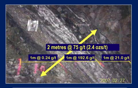
Sample of high-grade ore in mine: 2 metres wide @ 2.4 ounces per tonne.
