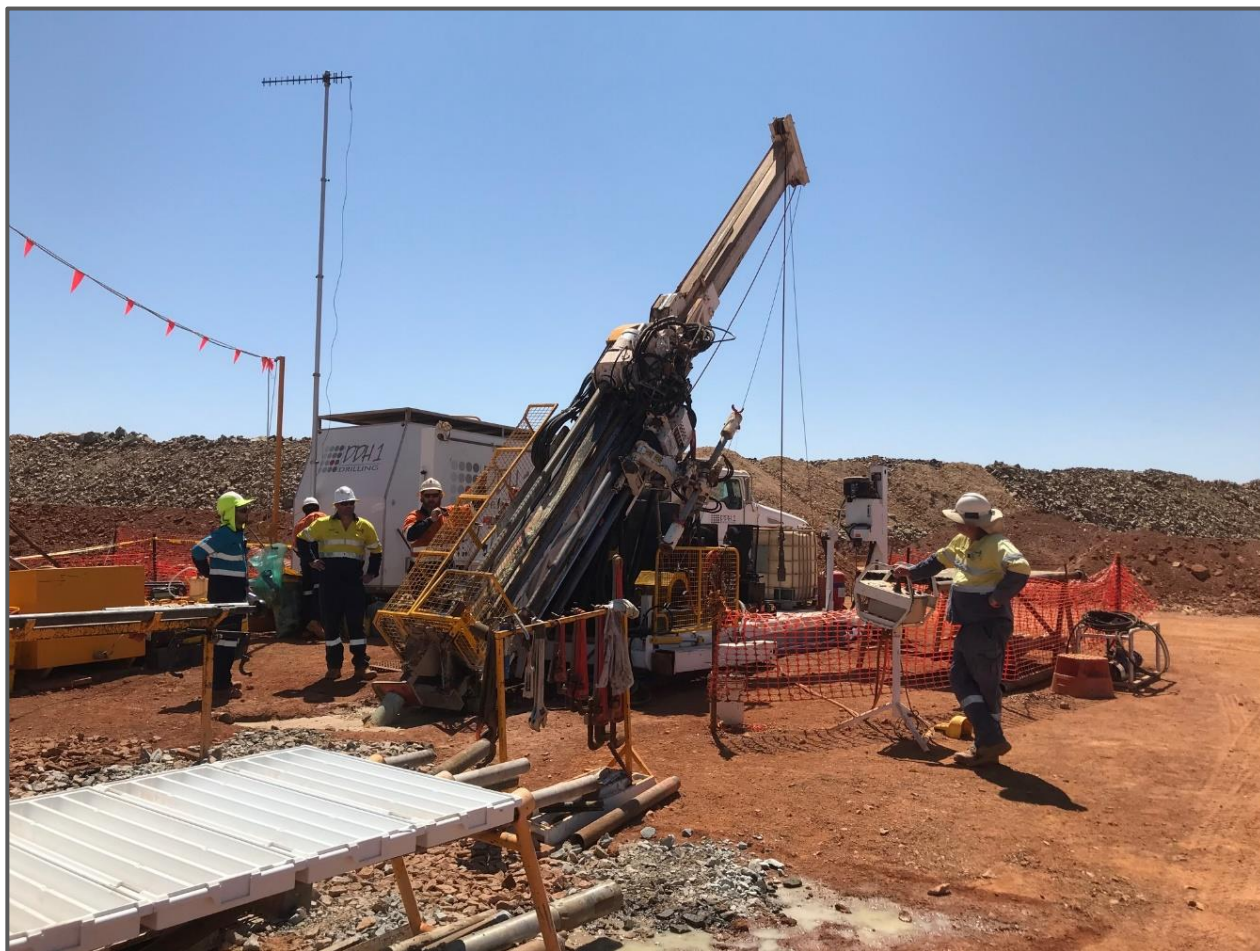
Figure 7: Eridanus diamond drilling – 2 nd hole at -42^{\circ}
