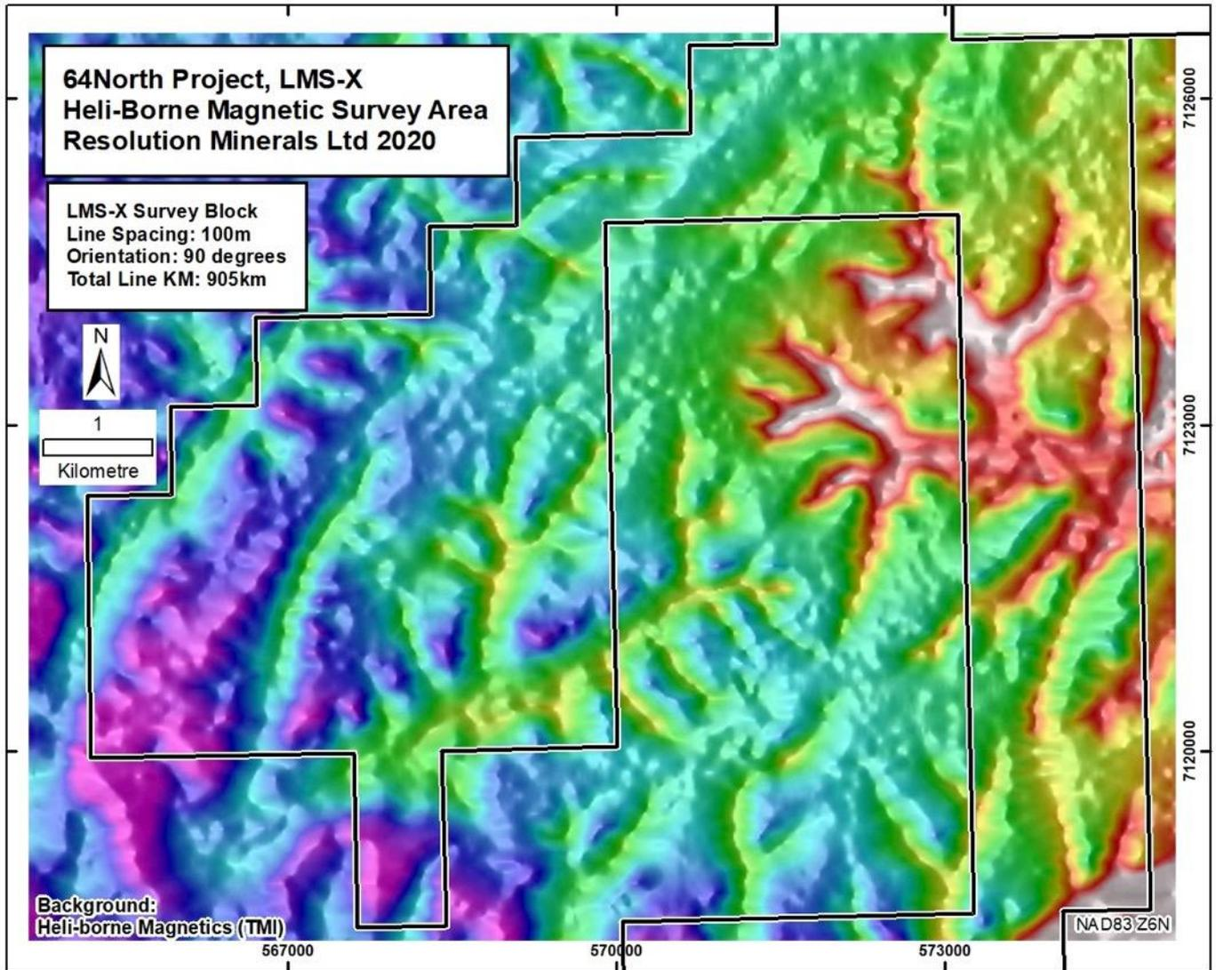
Figure 18 LMS-X Magnetic Survey (TMI), 905 line km, 100m line spacing, EW orientation, LMS-X Block, 64North Project Alaska.
