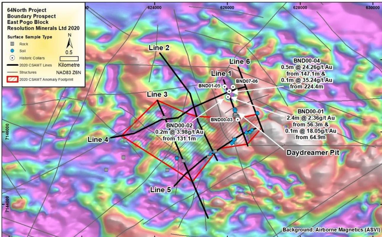
Figure 12 CSAMT survey lines with footprint defined for large anomaly. Follow up surface samples (assays pending) have been plotted (grey squares = Rock, blue circles = Soil). Background imagery is airborne magnetics (ASVI).
