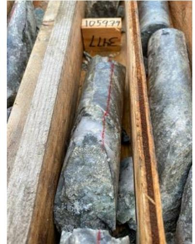
Figure 6 Quartz and sulphide veins at 1,060m Hole ID 20AU04 - typical of this hole.
