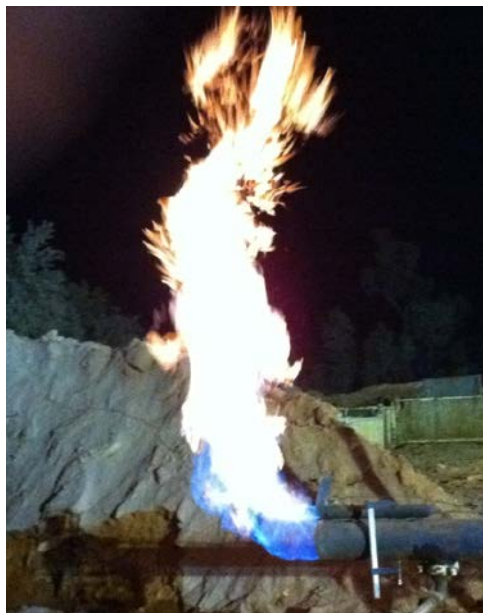
Figure 2 - Picture of gas burning from the end of the 8" diameter blooie pipeline, venting the Cow Lagoon 1 well
