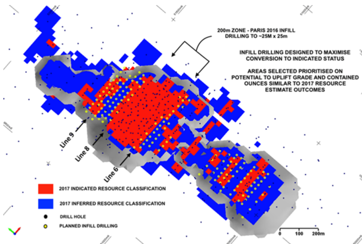
Figure 1: Shows the proposed 2020 infill program drill holes (yellow) across the Paris Resource – within the 2017 conceptual pit outline (grey). Drilling commenced on Line 8 and progressed toward Line 9 on 25m spacing.
