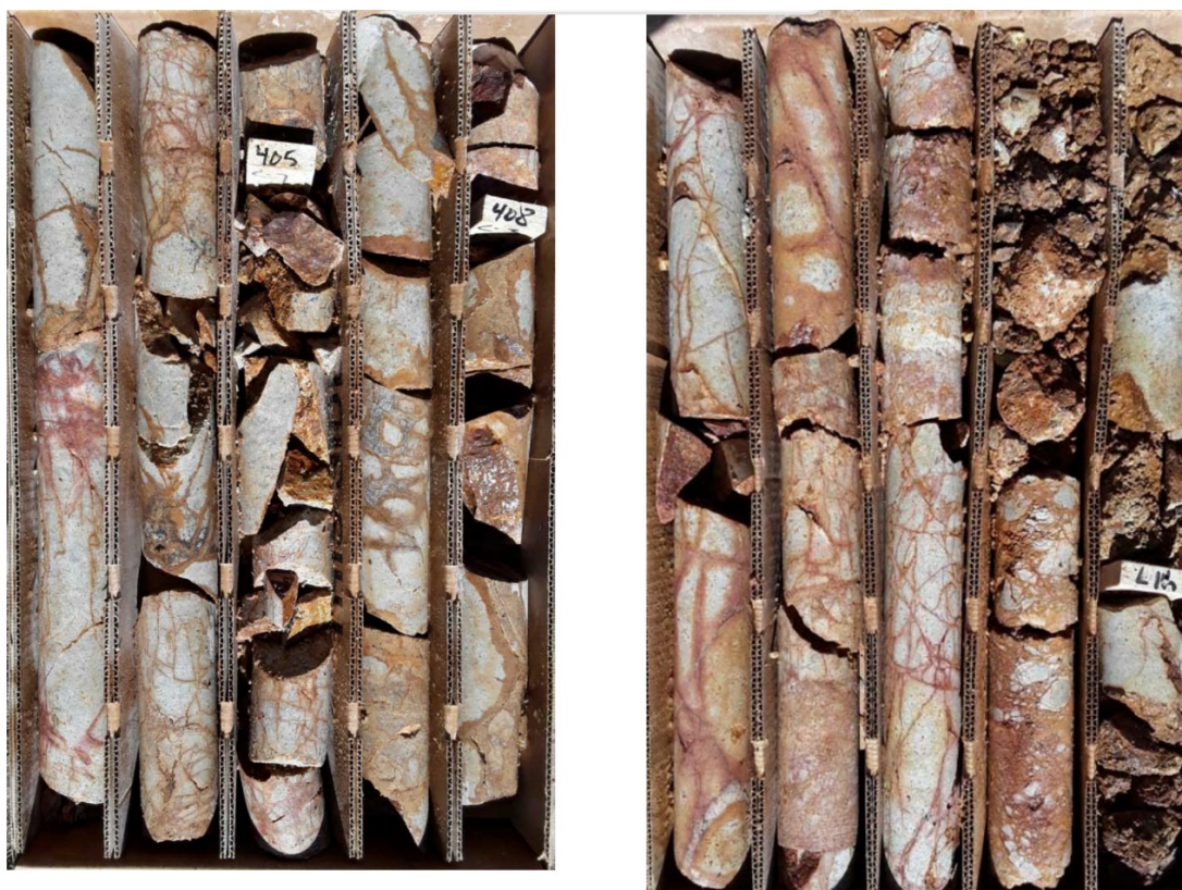
Figure 5. Highly fractured and oxidised intrusive rock in LCD-02 from 122.4m to 127.6m (401.5ft to 418.5ft); this “crackle zone” is above the targeted IP anomaly
