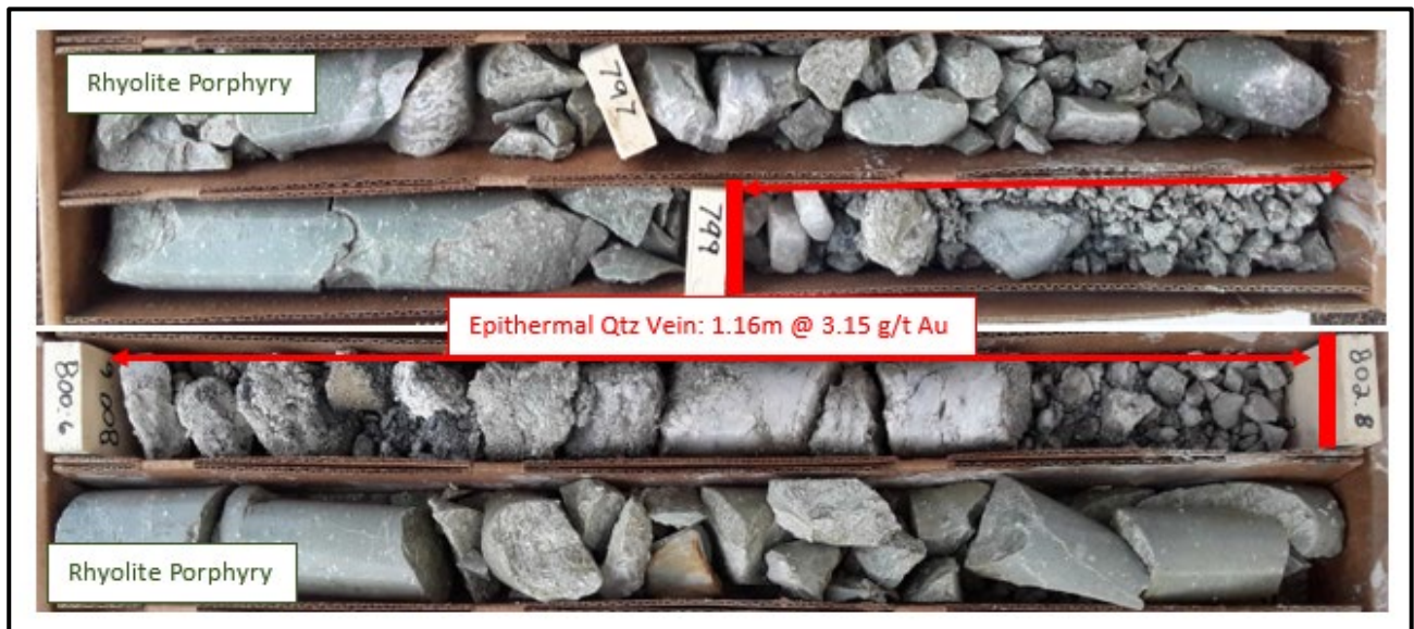
Figure 2: LCD_01 Drill core, showing epithermal quartz vein returning 3.2g/t Au (core block depths as shown in feet)
