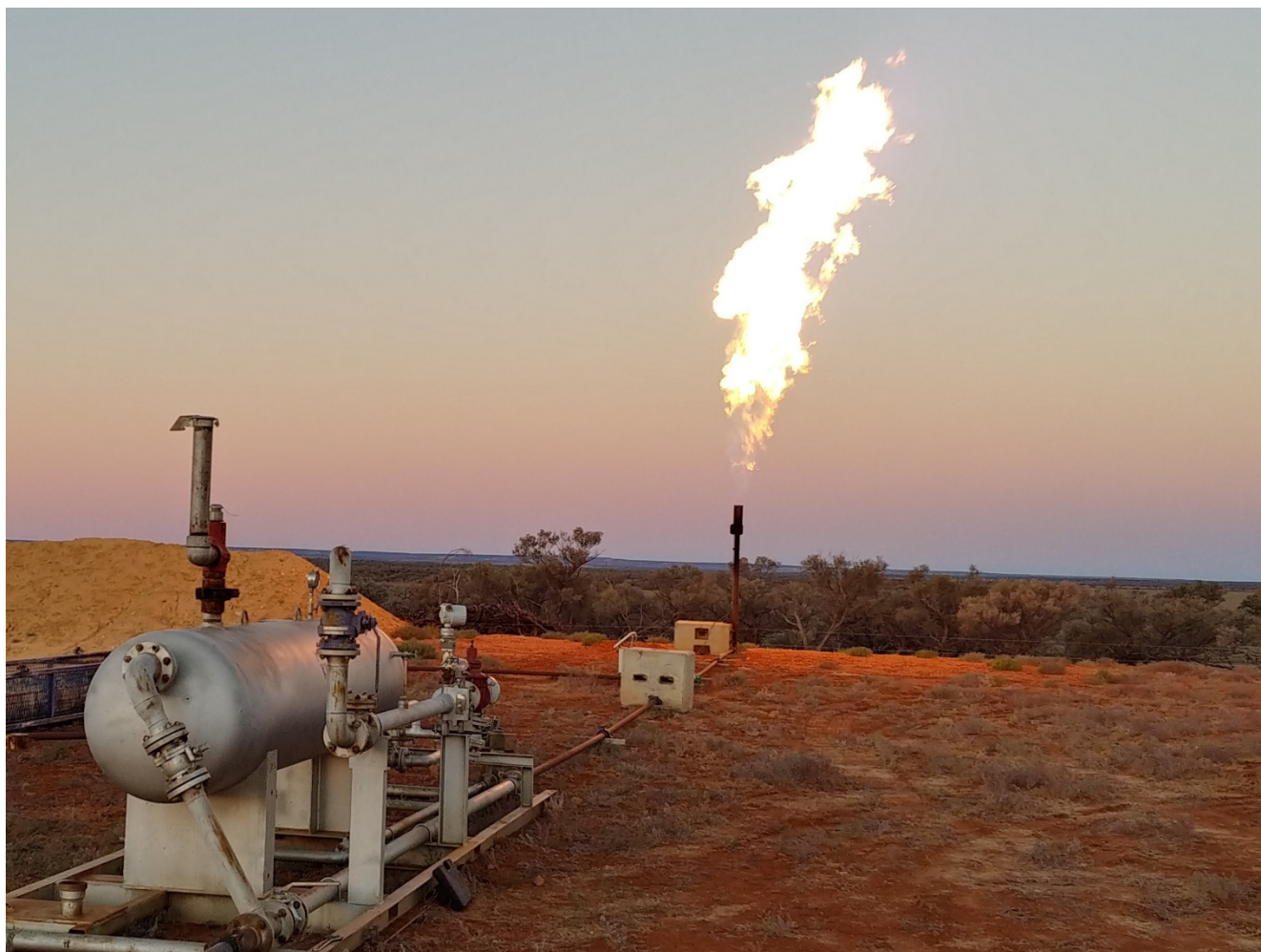
Flow testing at Windorah Gas Project in the Cooper Basin
