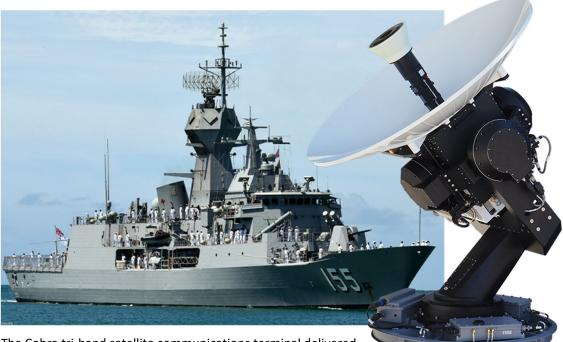
The Cobra tri-band satellite communications terminal delivered into the Australian Navy's Anzac frigate
