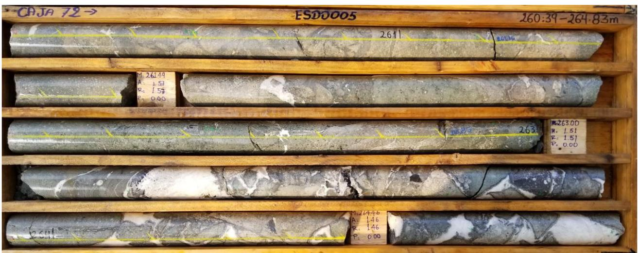
Figure 2: Drill hole ESDD005 from 260.5 to 264.8m showing argillic alteration, calcite veining and vein brecciation containing sphalerite (zinc sulphide) and galena (lead sulphide)
