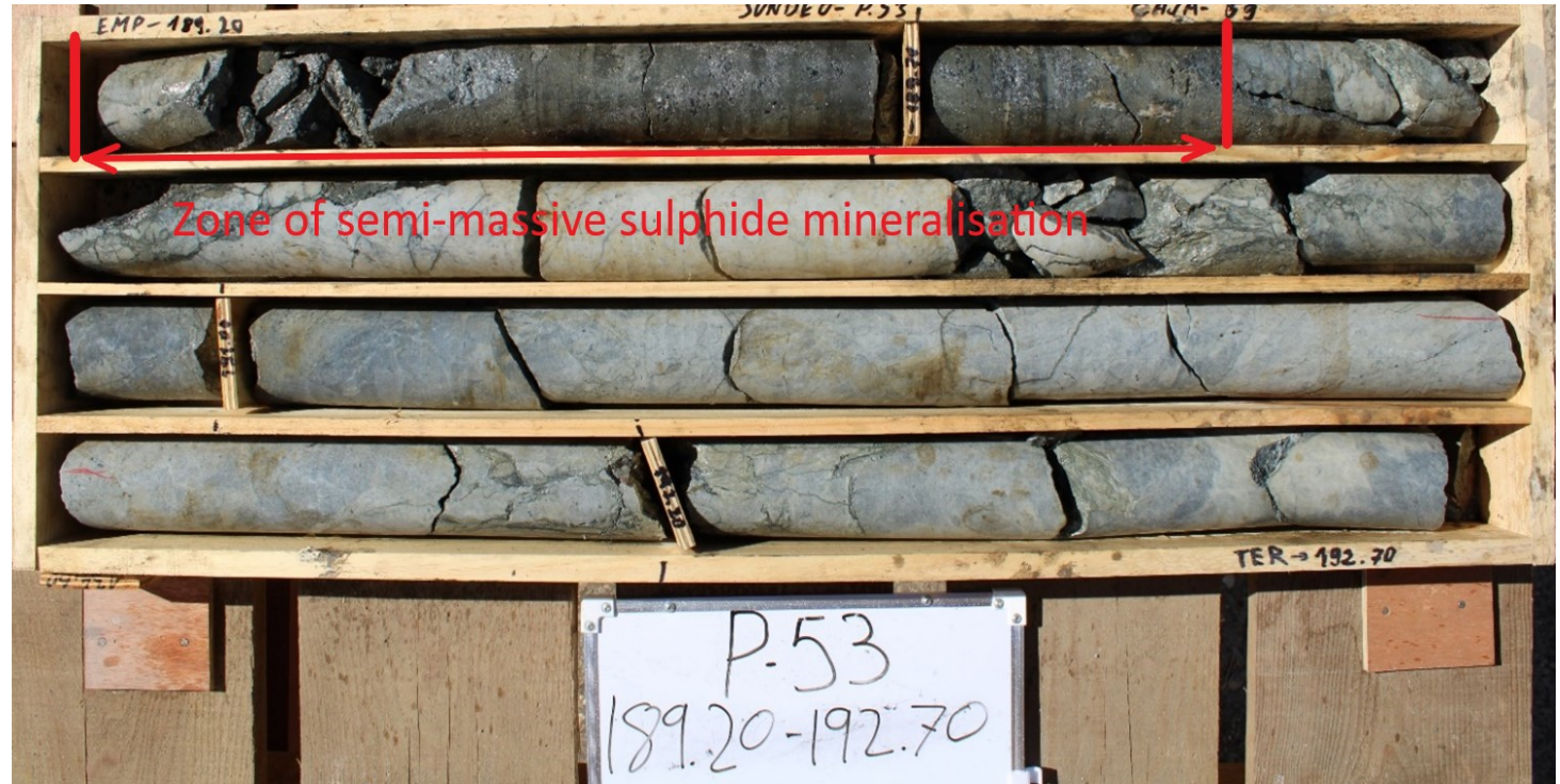
Exploration drill hole P53 depicting from semi-massive sulphide mineralisation from 189.2m – 190.2m
