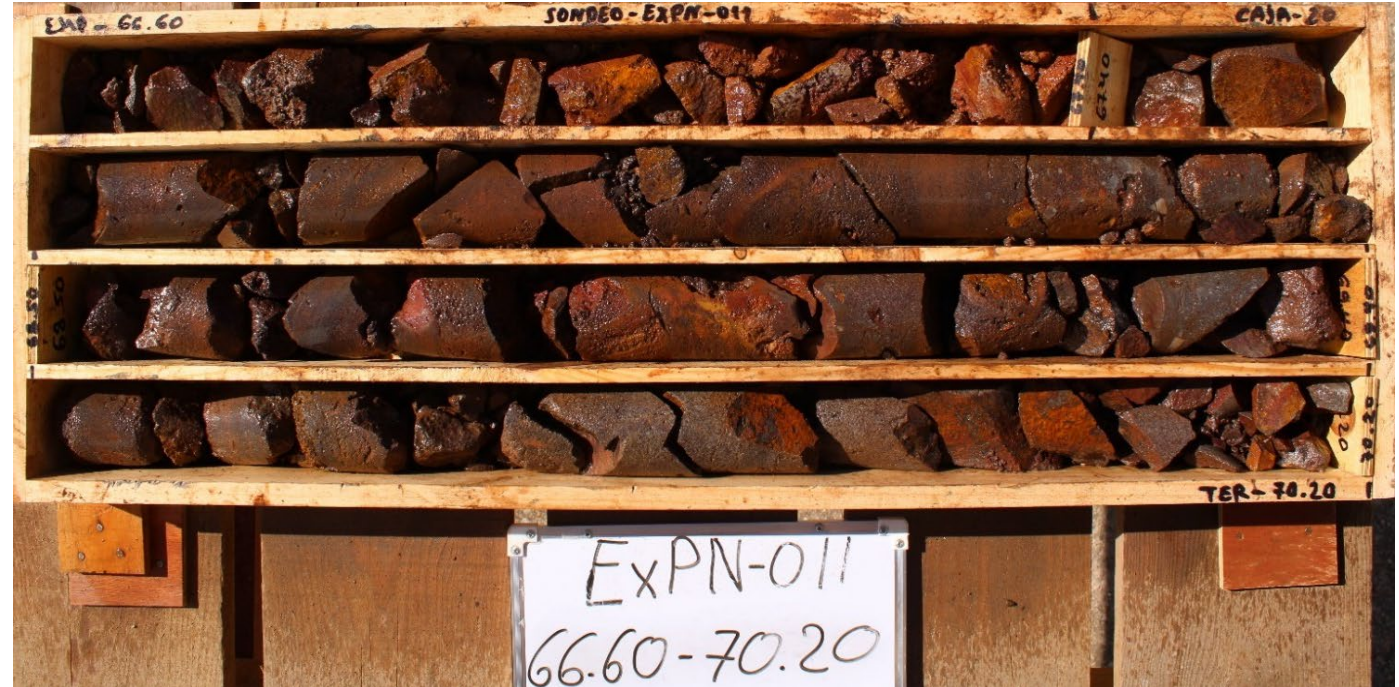
Expn_011 from 66.7m - 70.2m. Significant oxidation of sulphide mineralisation and textures typical of tin mineralised zones at Oropesa.
