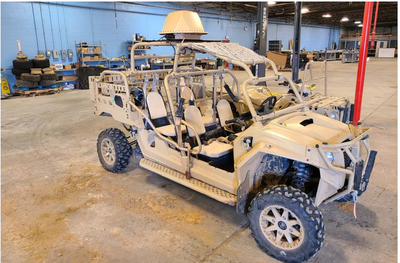
Image: DroneShield's on-vehicle DroneSentry-X™ system for detection and defeat of improvised threats
