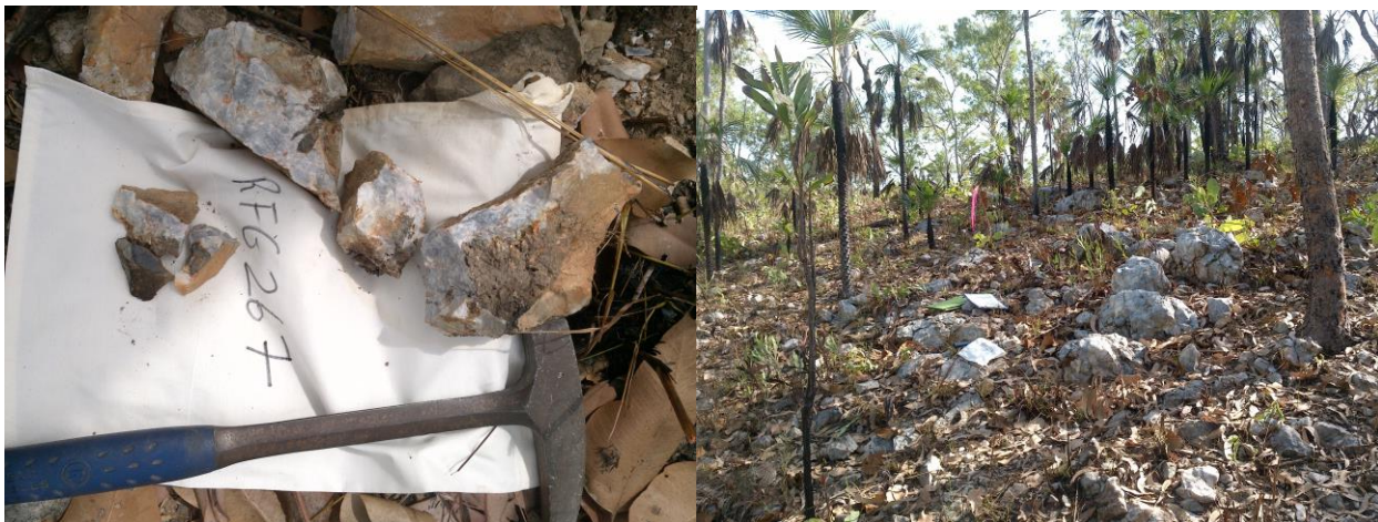
Figure 1. 20g/t Au rock-chip sample of vein quartz with iron oxides after sulphides (left). Quartz veins outcrop in the BBF Goldfield (right).
