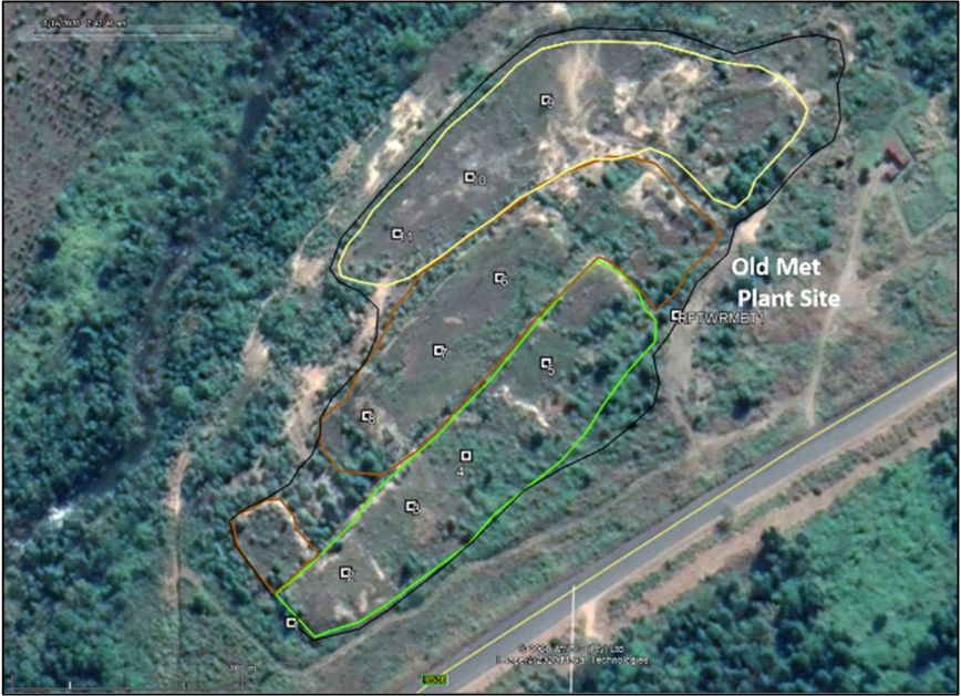
Figure 17: Rietfontein tailings sample localities. (Green=Top dump; Brown=Middle dump; Yellow=Bottom dump). RTFWRD1 is a sulphidic ore sample from the old ROM pad (av assay 13 g/t Au).
