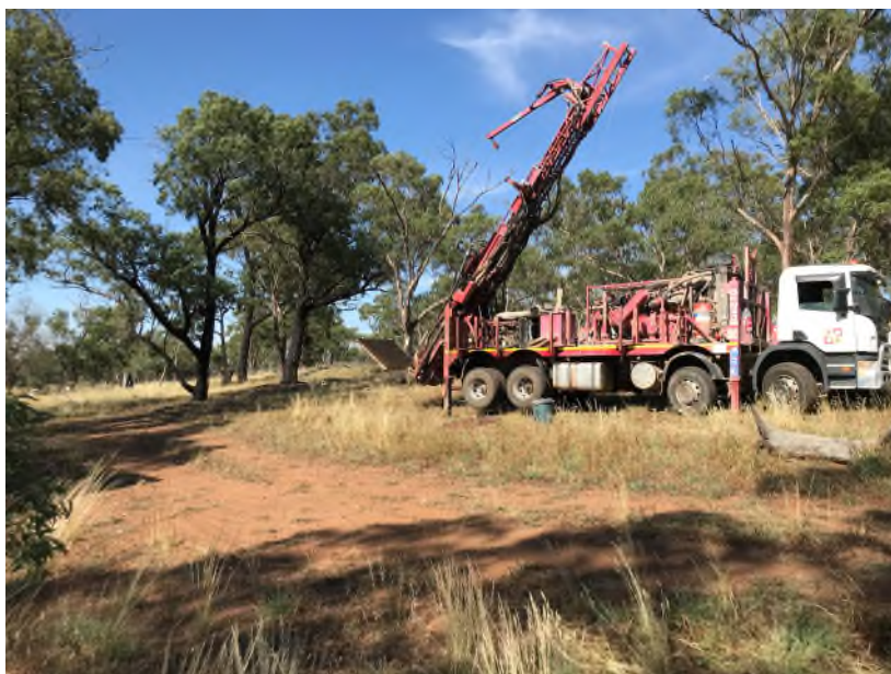
Figure 1 – RC drilling rig on site drilling Yalgogrin gold project
