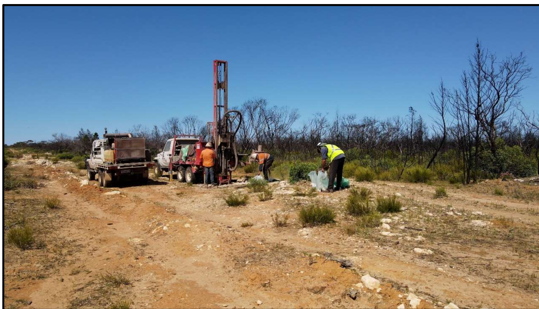
Figure 1: Air-Core Drilling at the Gibraltar Project (EL6506), South Australia
