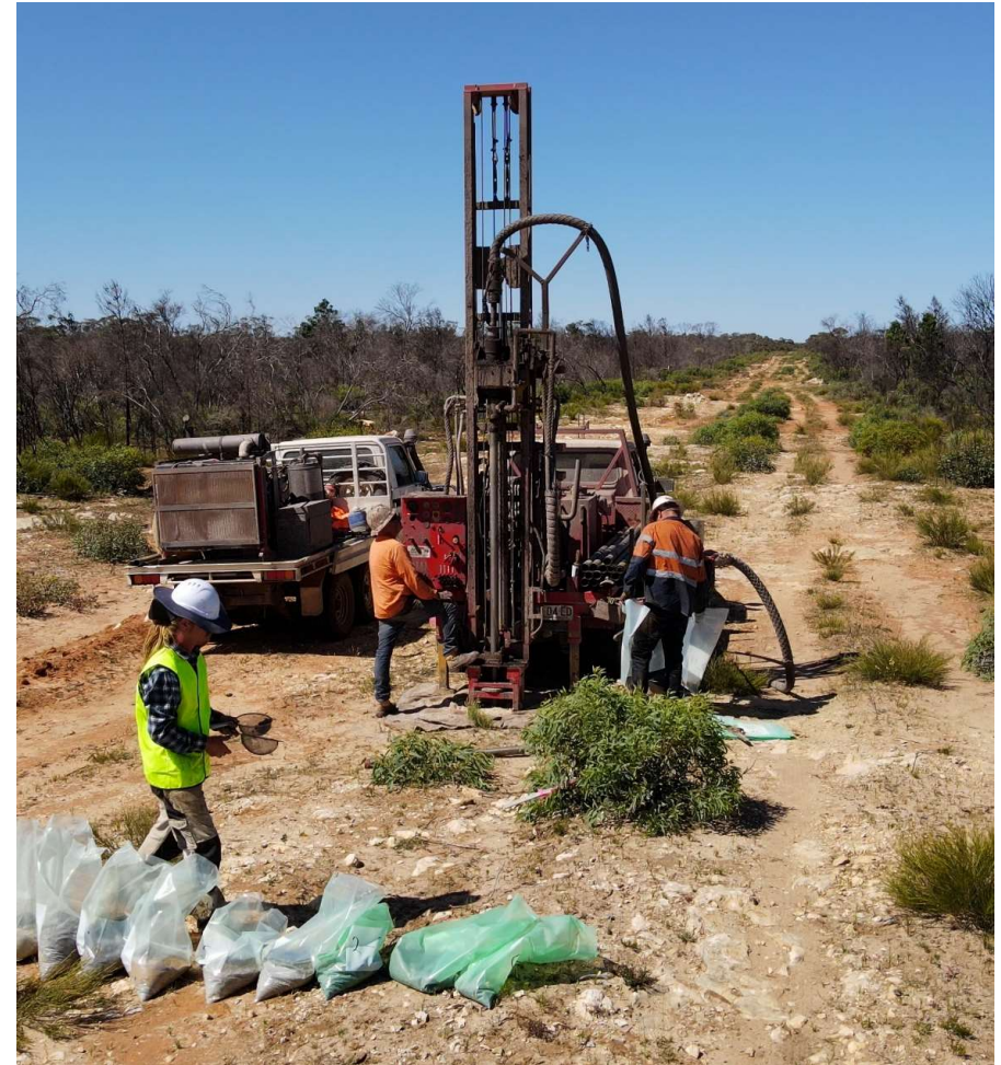
Oakdale's Gibraltar Kaolin - Halloysite Prospect – air-core drilling
