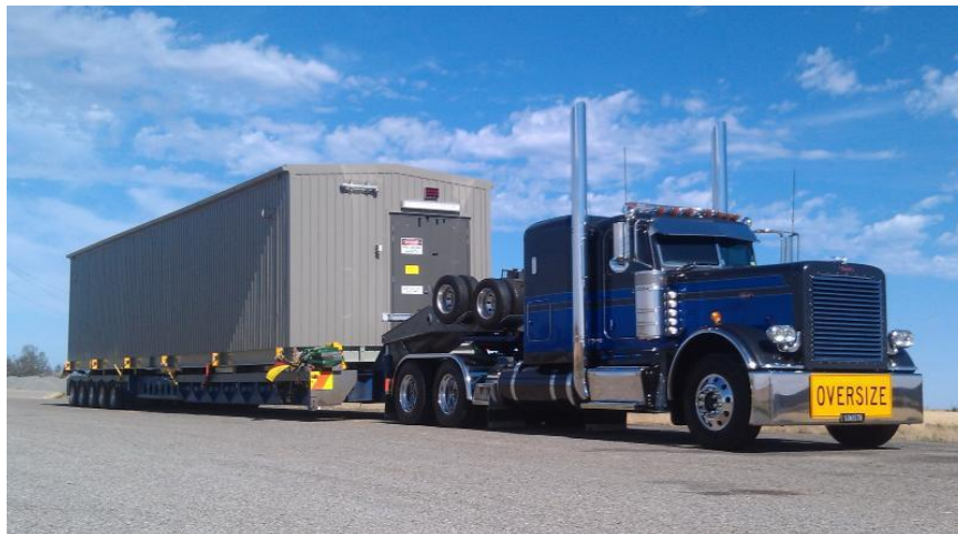
A Mayfield 45,000kg transportable switch room on route from Adelaide SA to Roma QLD for a major LNG project
