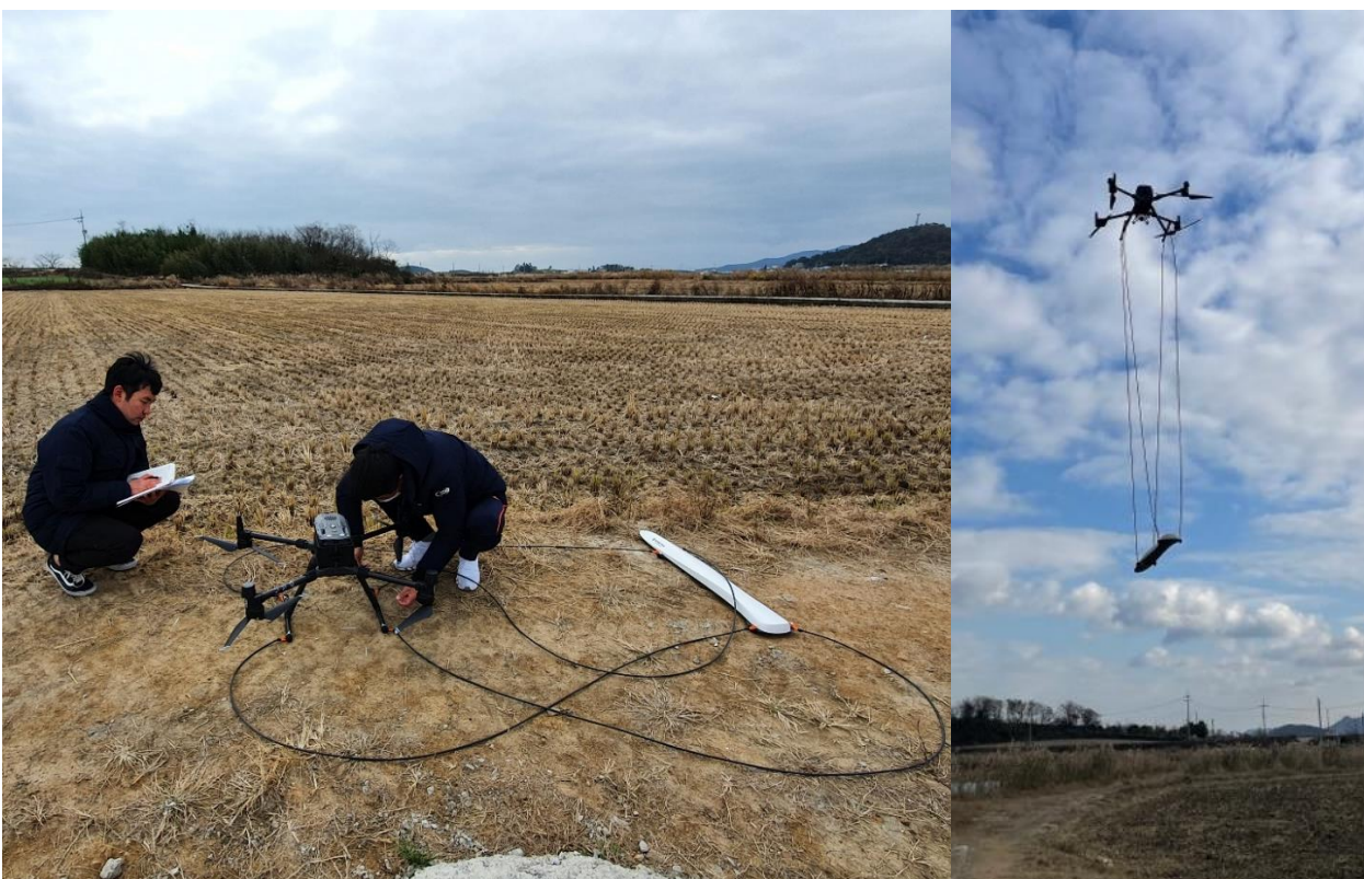
Photo 2 and 3 – Drone and magnetometer being set up (left) and in operation (right)
