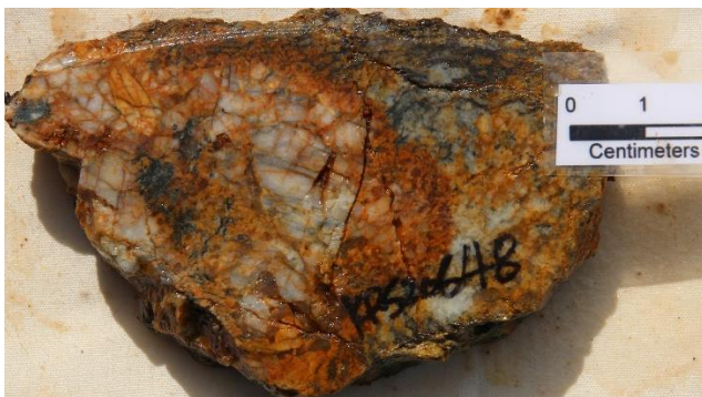
Photo 6 - Jeonpung Mine, Qtz-bt gneiss/schist hosted qtz vein with limonite-hematite oxidation, float. 6.7g/t Au, 1.6g/t Ag, 260ppm Bi, 273ppm Cu, 11ppm Pb, 146ppm W, 16ppm Zn. KRS206648.
