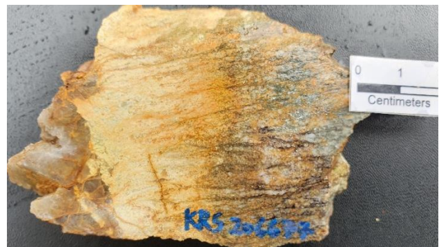
Photo 7 - Jeonpung Mine, Qtz-bt gneiss/schist hosted qtz vein with limonite-hematite oxidation, outcrop. 4.66g/t Au, 0.6g/t Ag, 167ppm Bi, 52ppm Cu, 13ppm Pb, <10ppm W, 12ppm Zn. KRS206677.
