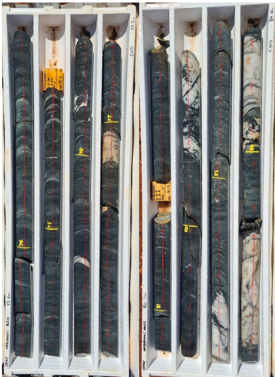
Figure 5: Diamond core from MZDD001 73.6m-77.3m and 80.9m-84.4m showing multiple gold bearing quartz sulphide veins within the ~8m wide Metzke's shear zone with visible gold seen at 76.9m, 83.5m and 84.2m
