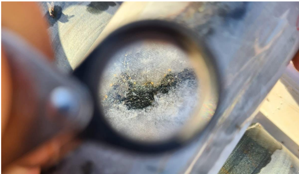
Figure 1: Image of visible gold through a hand lens from MZDD001 hosted within a narrow laminated saccharoidal quartz-sulphide vein.
