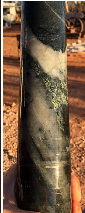
Figure 6 (R): Image of one of the saccharoidal quartz-sulphide veins from 53.6m to 53.8m LMDD001 drilled at Longmore's Find
