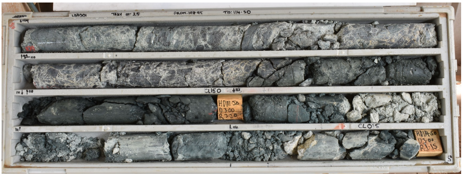
Figure 5: LDD001 from 109.0-114.5m. Polymictic breccia including porphyry clasts
