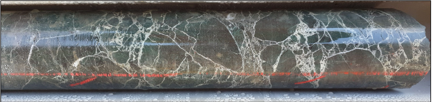
Figure 1: LDD001 core showing breccia with quartz-carbonate stockwork infill
