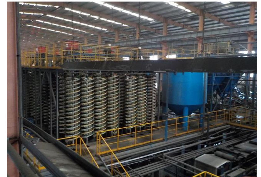
* Astron's spirals, developed specifically for separation of fine mineral ores.
