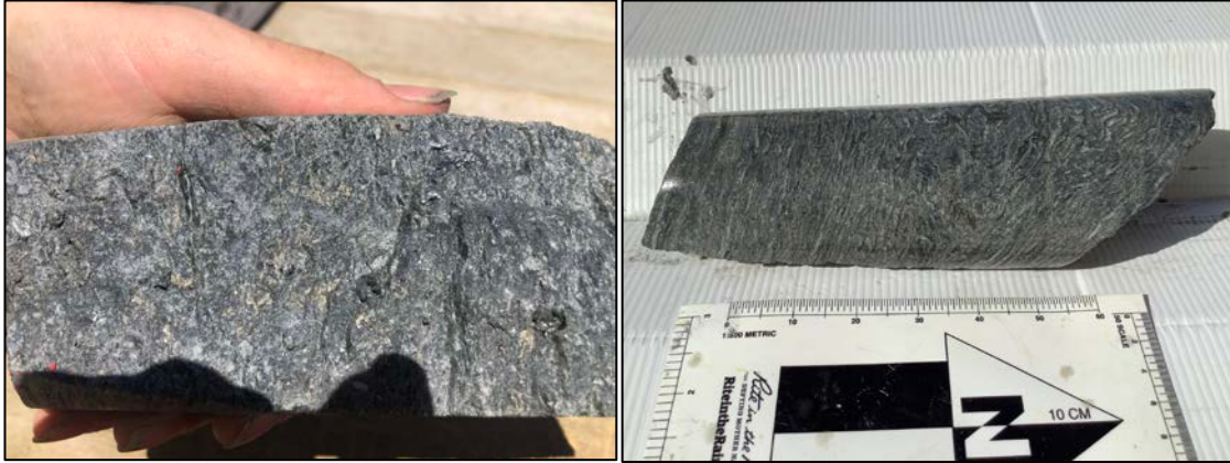
Figure 3: Drillhole CBN0005 at 88.1m, showing visible silica-carbonate-pyrite +/-arsenopyrite +/-sericite alteration. In the photo on the left, a fracture surface exposes sulphide mineralisation with pyrite and probable arsenopyrite which can be seen throughout the rock. Pale silica carbonate alteration is also visible. In the second photo the outside of the core shows strong foliation and micro folding associated with local shearing which has allowed the mineralising fluids to move through the schist.
