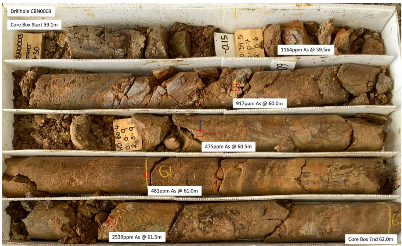
Figure 2: Drillhole CBN0003, showing regular portable XRF analysis at 0.5m locations with consistently elevated arsenic levels, ranging from 475ppm up to 2539ppm across this 2m section of core. The core is oxidised, brecciated and sheared.
