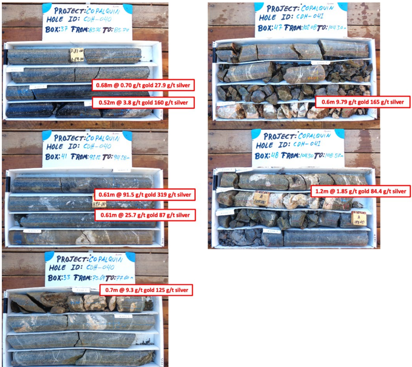
Figure 1: Core photos for hole CDH-040 and CDH-041 intercepts. Well milled breccia clasts in dark coloured silicified matrix. Highest grades occur along margin of rhyolite dike.
