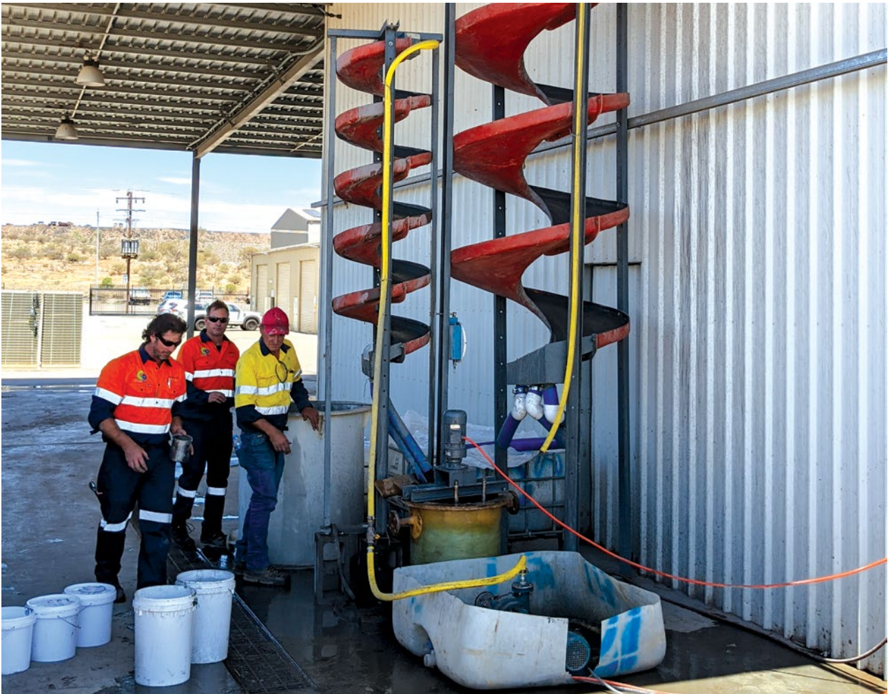
Figure 3 – Pilot Plant Progress Update – Concentration Circuit – preliminary testwork has begun
