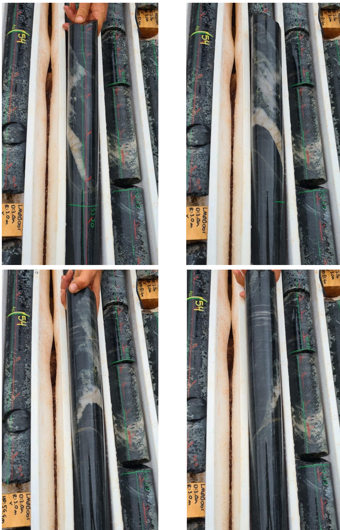
Figure 3: Four images showing the quartz-sulphide vein not cutting across the core, indicating a subparallel orientation to the drill direction, and evidence of post mineralisation folding and deformation.
