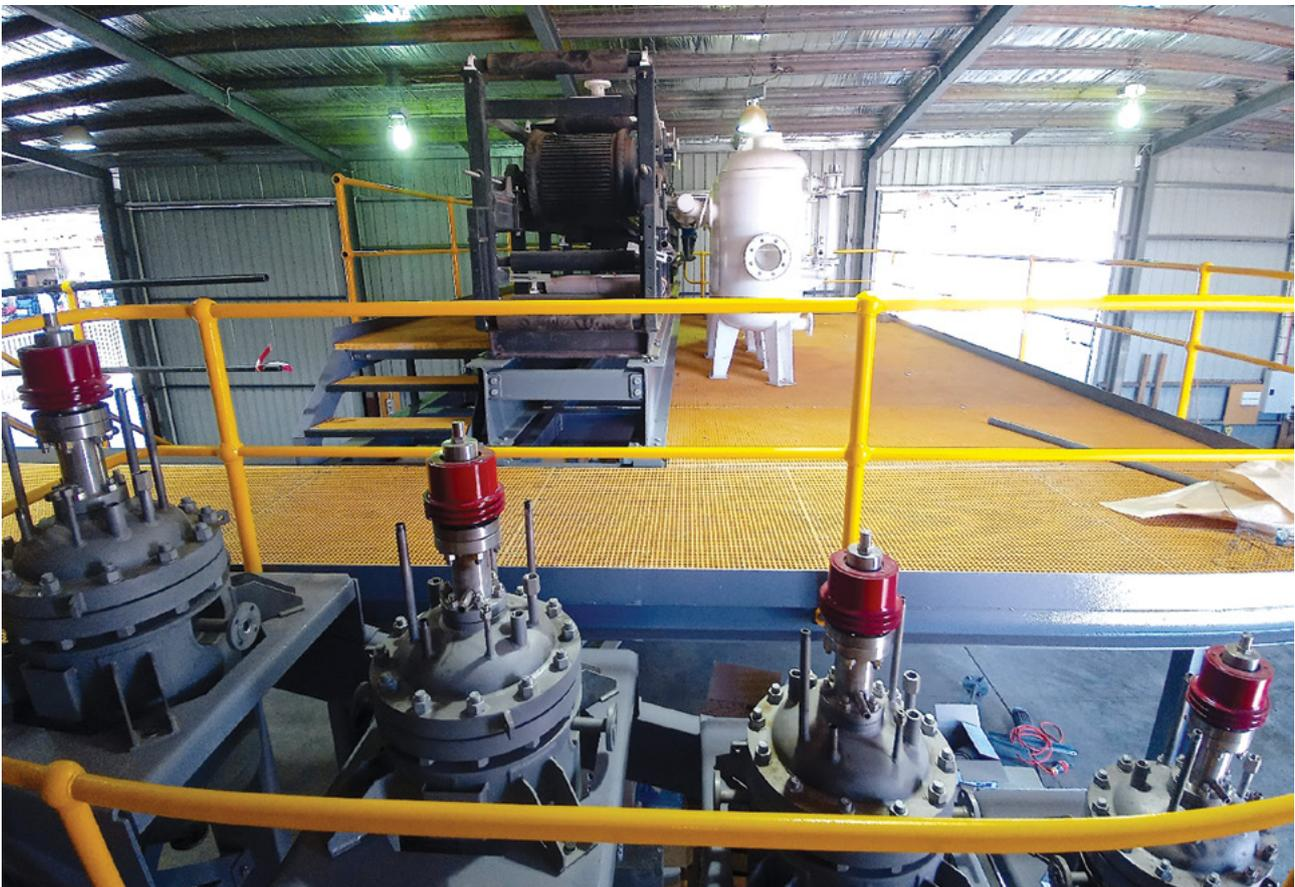
The Pilot Plant will test COB's process technology on a continuous basis. The throughput rates are nominally 1–2 t per hour for the concentrator circuit and 100–150 kg per hour for the leaching circuit. COB will process up to 90 t of ore (RC Chips) through the plant, using existing samples collected in previous drilling campaigns.
