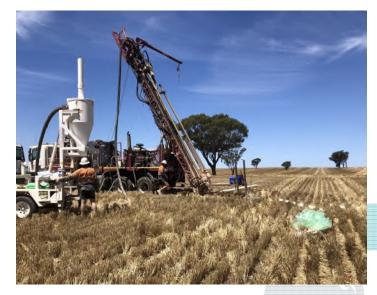
Figure 1 – RC rig on site drilling at the Harry Smith gold project
