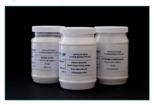
Photo: Samples of three products produced from Rhyolite Ridge Ore: Lithium Hydroxide, Lithium Carbonate and Boric Acid
