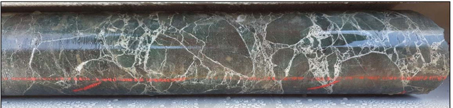
Figure 5: LDD001 core showing breccia with quartz-carbonate stockwork infill
