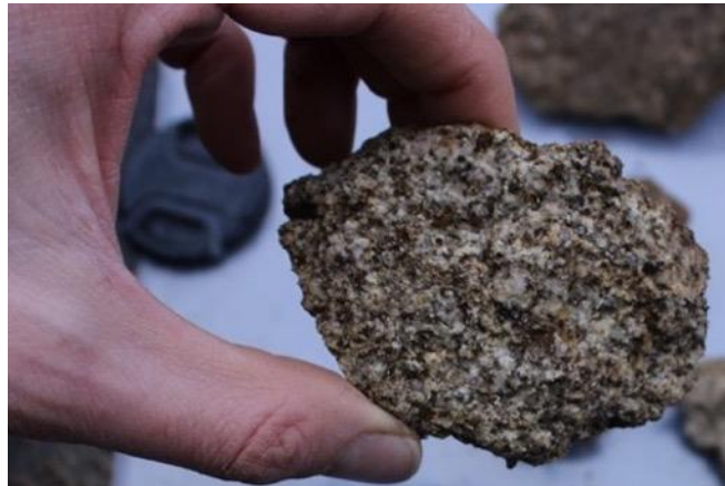
Figure 8 Quartz-feldspar-biotite granite samples from road cut 20AT001T. Sample 707517 (left) assay returned 1.63g/t Au from 66-67m and includes 1-6mm wide quartz veins (sheeted vein sets). Sample 707529 (right) assay returned 1.89g/t Au 78-79m.
