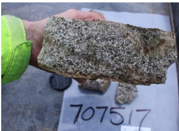
Figure 8 Quartz-feldspar-biotite granite samples from road cut 20AT001T. Sample 707517 (left) assay returned 1.63g/t Au from 66-67m and includes 1-6mm wide quartz veins (sheeted vein sets). Sample 707529 (right) assay returned 1.89g/t Au 78-79m.
