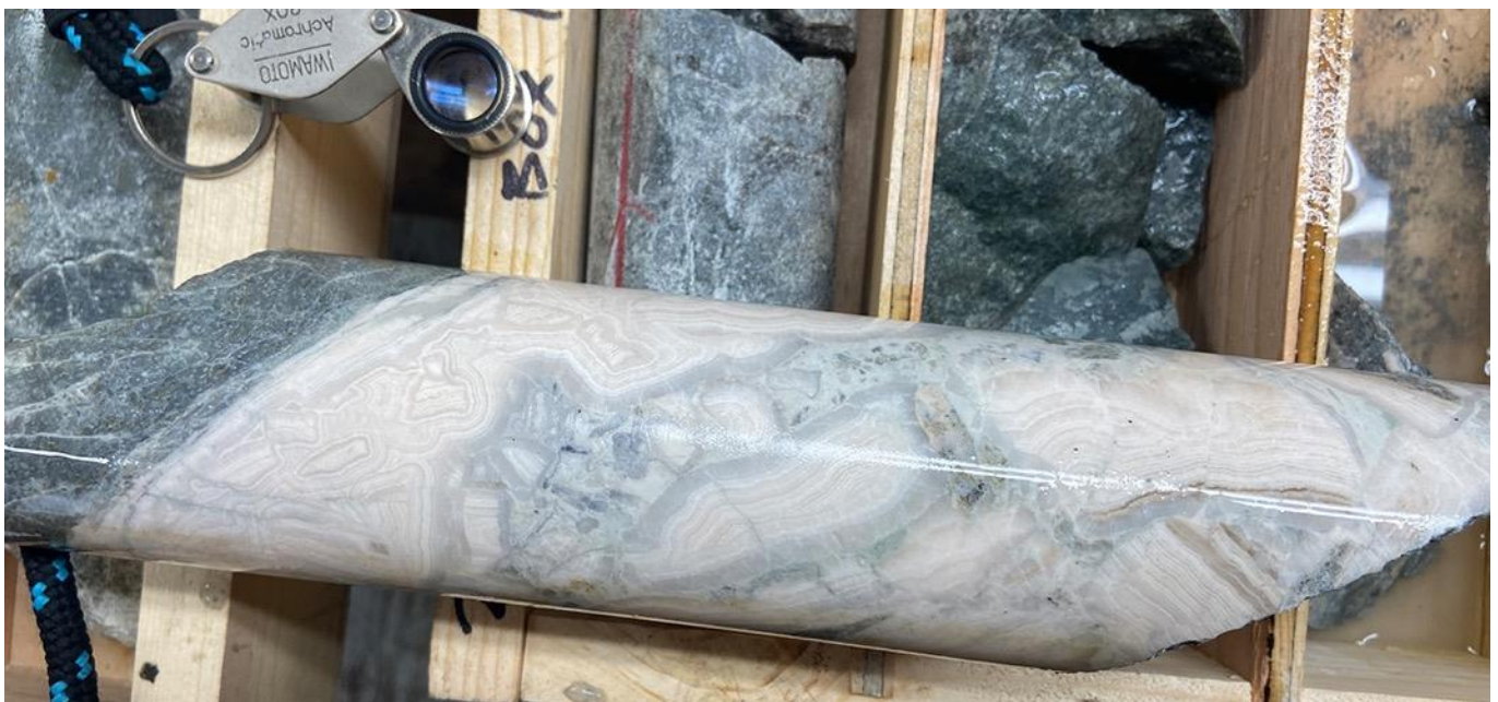
Figure 10 drill core (HQ) interval 212.35 – 212.50m hole 20AU09. Example of a brecciated colloform quartz vein “dilational zone”.
