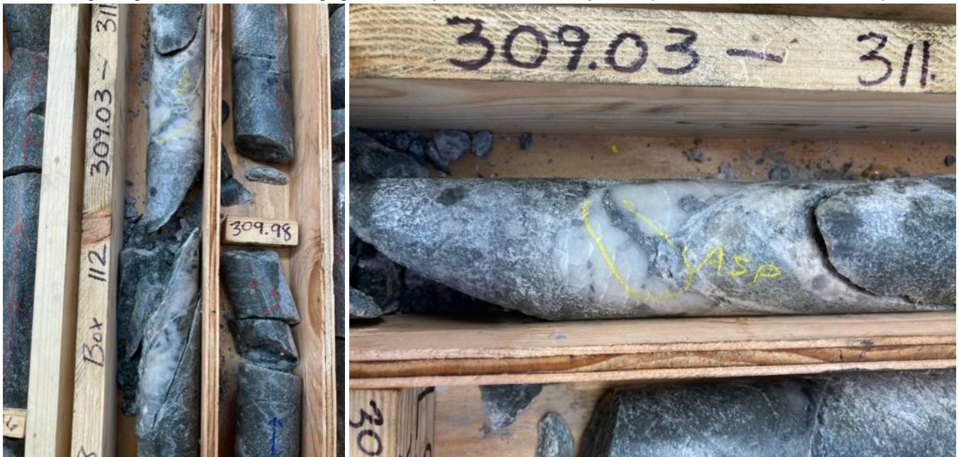
Figure 9 Example of a quartz-sulphide vein “dilational zone” intersected in hole 20AU08. The photo on the left is an interval of NQ drill core from 309.18 - 309.78m. The photo on the right is a zoom in on the interval 309.18 - 309.38m with an arsenopyrite vein cross cutting a quartz vein highlighted with yellow markings.
