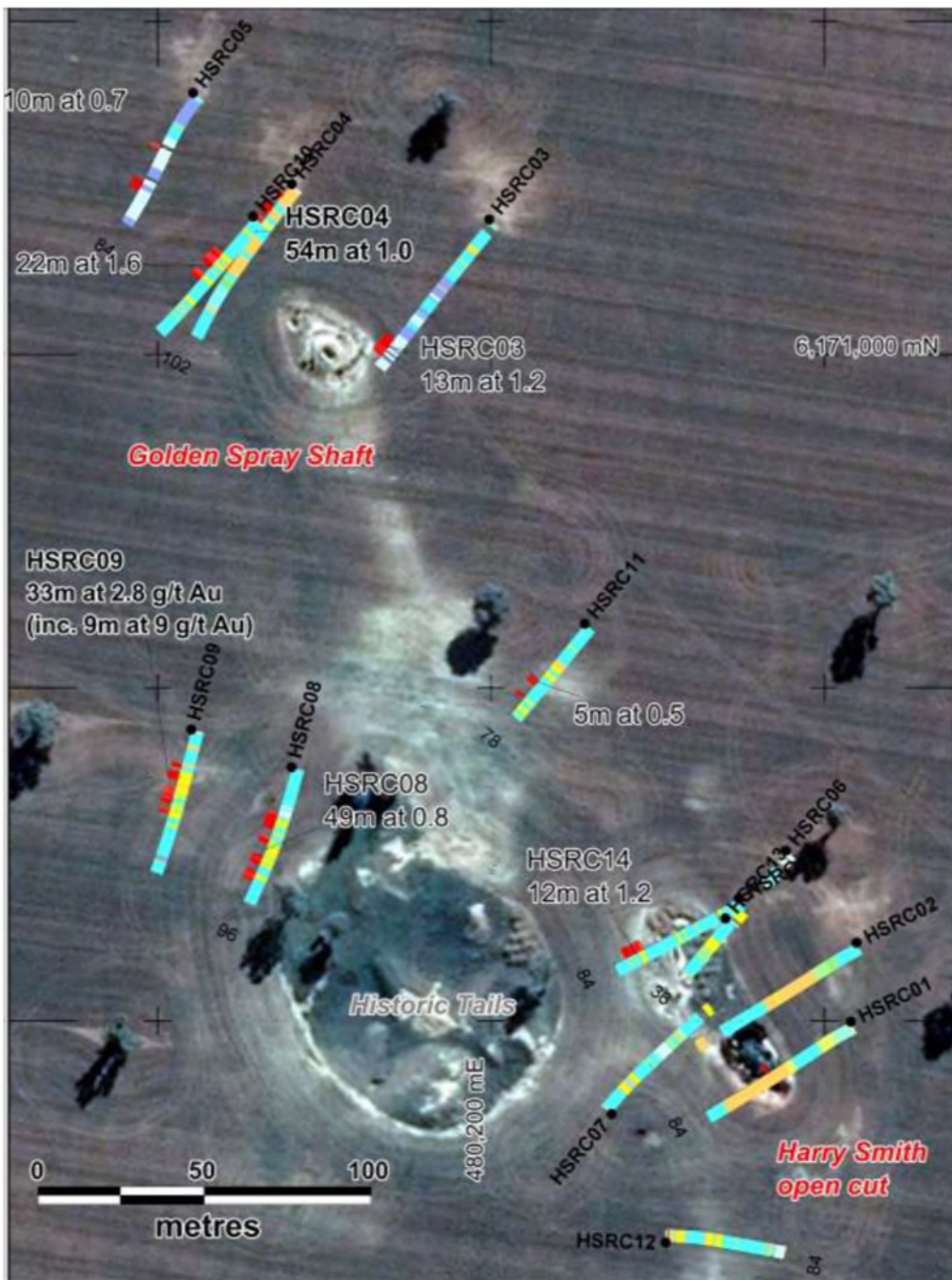
Figure 4 - Thomson Resources drill intercepts at Harry Smith (red bar graph shows gold intercepts greater than 0.5 g/t Au, the other side shows that rock types are mostly siltstone or sandstone with yellow indicating quartz veining)
