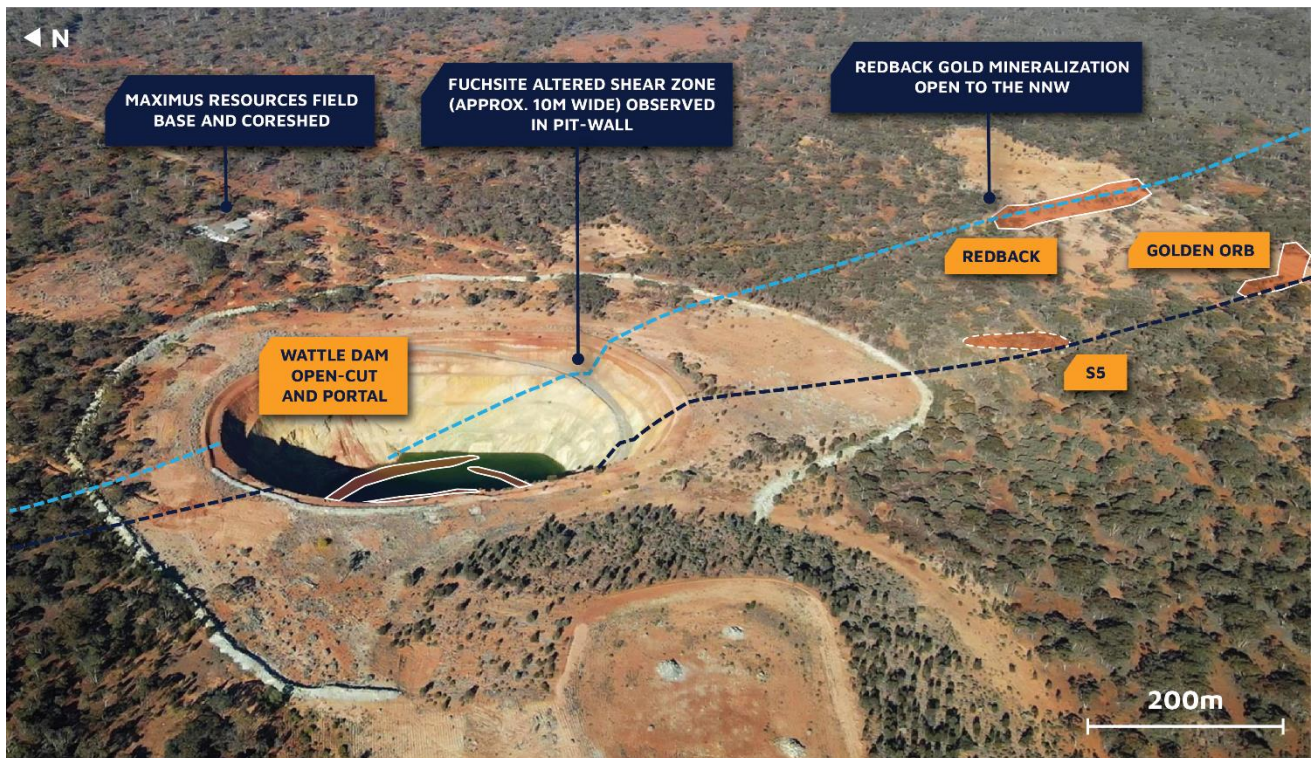
Figure 2 - Aerial image of the Wattle Dam open-cut and southern prospects illustrating the relative location of the S5 prospect.
