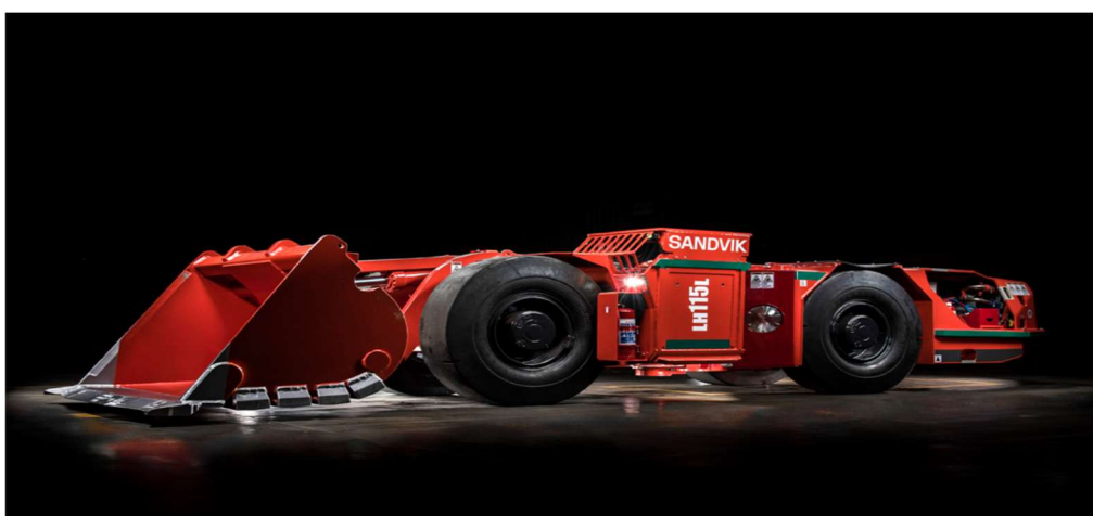
Figure 4: Sandvick low Profile LHD – At a height 1.6 m designed for operation in narrow-reef drill drives
