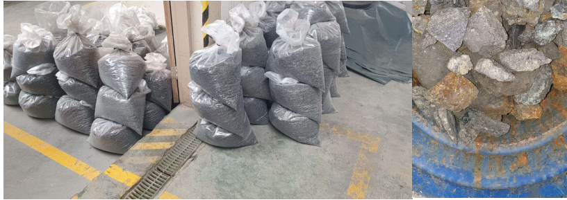
Underground ore samples from mine face 20+ mm sample size (5 tons of sample collected from underground mine)
