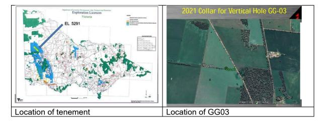
Through the interpretation of the Geophysical data a vertical hole will be drilled at location GG-03. This was chosen due to a focused strong target area based on modeling from the geophysical work conducted in Jan 2020.
