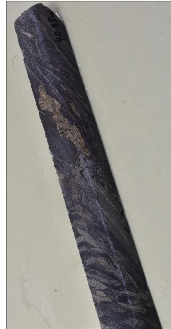
Recent NMR drilling campaign intersects schistose porphyry with bands of massive pyrite , LDD002 40.85m
